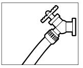
**Step 3** Connect garden hose to the cold water source and turn water on completely.
